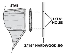
13. Use a leftover piece of 3/16" sq. hardwood to make a drill jig for the stab wire holes. Drill two 1/16" holes in the jig using the spacing shown on the plan. The jig will insure the holes are drilled in exactly the same location in each stab half. Using the jig, drill two holes in the stabilizer root ribs. Be careful to drill the holes centered in the rib and parallel to the stab surface.
